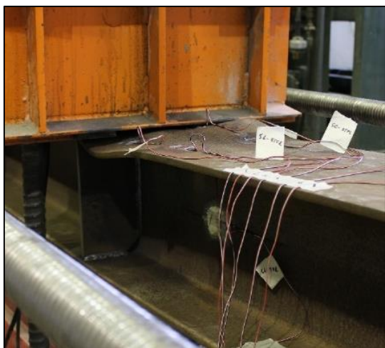
Figure 5.6 Localized failure of base section flange
