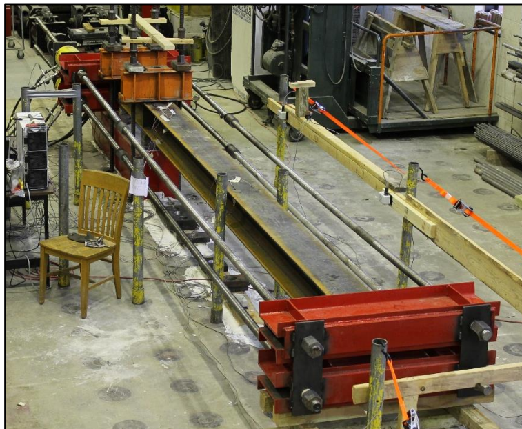
Figure 5.26 Non-deteriorated pile bent test
