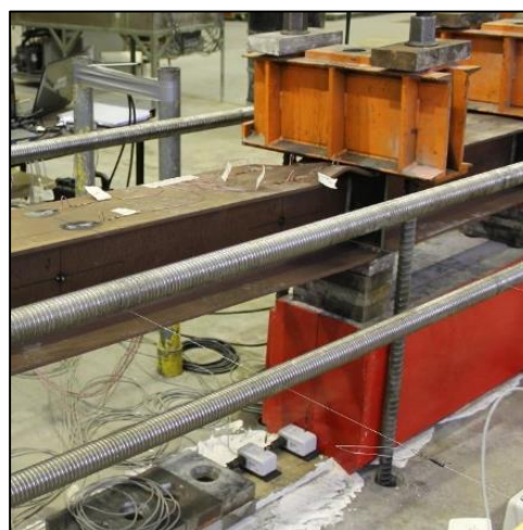
Figure 5.5 Buckling of base section top flange
