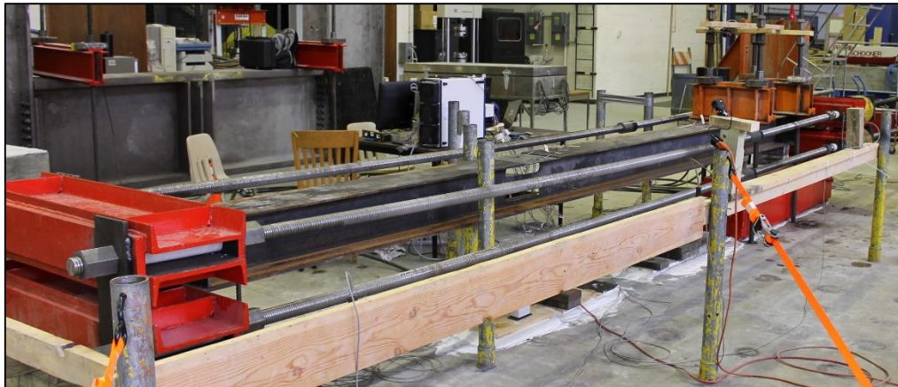
Figure 5.33 Deteriorated pile bent test
